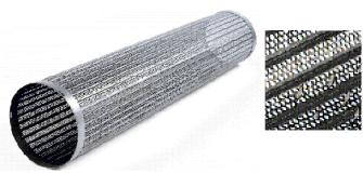
**FUNLSIZER®** This patented cylinder is the latest in technological design. The perforations are funnel shaped round holes. The funnel design upends the grain directly into the hole and either allows passage through the hole or rejects the grain and passes it down the cylinder. The funnel style holes are available from 13/64 inch (5.2mm) to 23/64 inch (9.1mm) in diameter. Best for separating large particles by width.
