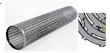
TRI-BAR - The Carter Day Tri-Bar slotted cylinder can double the cylinder capacity depending on slot width. The Tri-Bar operates by using a triangular shaped wire, instead of punched slots, producing more open area. Rigid construction maintains opening tolerance longer. Slot widths are available in sizes from 2.5/64 inch (1mm) wide to 36/64 inch (14.3mm) wide. Best for separating particles by thickness with high capacity.
