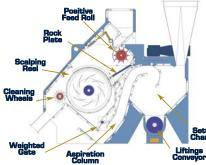
The 24" Low Profile Scalper features scalping and sifting in a single machine to provide a high capacity method for removing roughage and fines in a single
